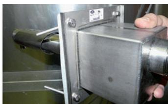
View of the bolts inserted in the support flange
