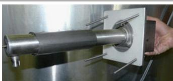
Insert the gasket and rest it against the support flange; insert the fastening bolts to secure the support flange
