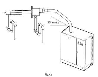
Nota: The adapters and steam hoses shown above are available as options. The "P" drains are not provided as part of the ultimateSAM system.
