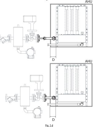
The pipe x is used to pass through the insulating panel on the AHU.
