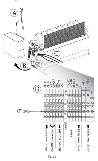
**Note**: to avoid unwanted interference, power cables should be kept separate from probe signal cables.
