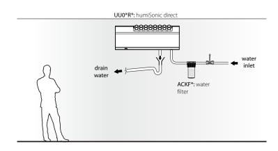
Ideal for small humidification loads (0 to 20 l/h) and where compactness, low noise and short absorption distances are required. Ease of droplet absorption and low noise make it ideal for comfort applications in public places. Its compact dimensions and high performance mean it can be used
