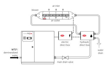
Suitable for managing medium and high humidification loads. The possibility of up to six independent zones, and a wide range of sizes (up to 1000 l/h), make this solution ideal for retrofits in industrial environments, where traditional ducted humidification is not possible.
