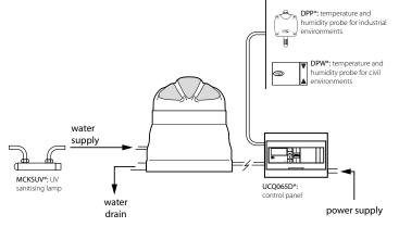
Stand-alone spinning disk humidifier available in sizes from 1 l/h to 6.5 l/h. Simple and efficient solution for cold stores or places where precision is not required and operating conditions are extreme.
