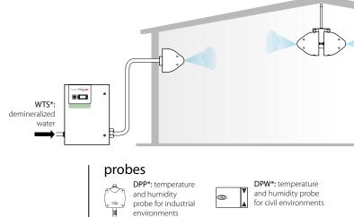
Designed for medium-sized industrial environments, combining maximum reliability with low operating costs. The electronic valves fitted inside the cabinet are used to manage the blowers and make the system easier to install, adapting to any context, even the most complex ones. The unit can be managed on a local network via webserver, and comes with the most common communication protocols: Modbus®, Bacnet™ via Ethernet and RS485.
