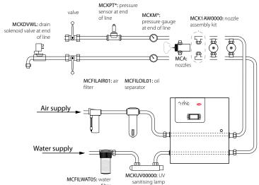
Compressed air and water humidifier, the ideal solution when a compressed air system is already available in the building, as is often the case in the industrial sector. The main target applications are printing, textiles, wood industries and food cold stores. The humidifier can communicate via Modbus®, LON, TCP/IP and SNMP using a special additional card.
