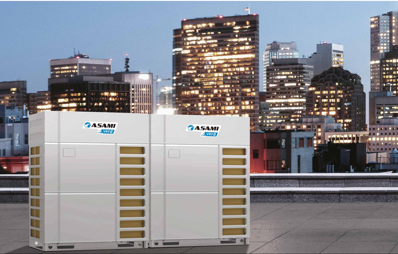
AMV6 heat pump multi VRF unit adopts air-makeup enthalpy-adding compressor, brand new dual zone heat exchanger and CAN+ system control proposal. Seasonal energy efficiency of the whole is greatly improved, with SEER and SCOP improved by up to 20% and 30% respectively.
