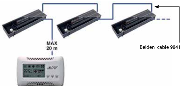
ONE CONTROL FOR MORE UNITS (20 UNITS MAX.) (MAXIMUM TOTAL LENGTH OF THE CONNECTION CABL = 800 m)
